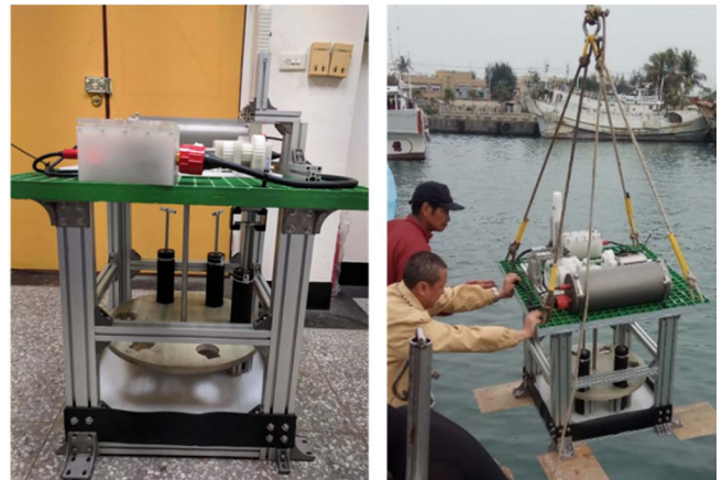
Fig. 12 Self-sustaining version of IUT prototype APC (left) and functional test of IUT prototype APC in Kaohsiung harbor (right).
