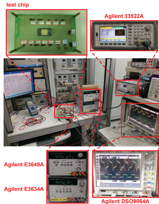
Fig. 5. Measurement site setup
