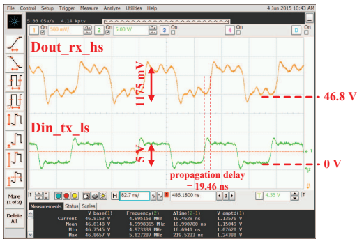
Fig. 8. Waveform of digital pulse at 5 Mbps, 50 V
