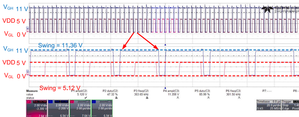
Fig. 20. Measurement result of V_{GH} and V_{GL} .
