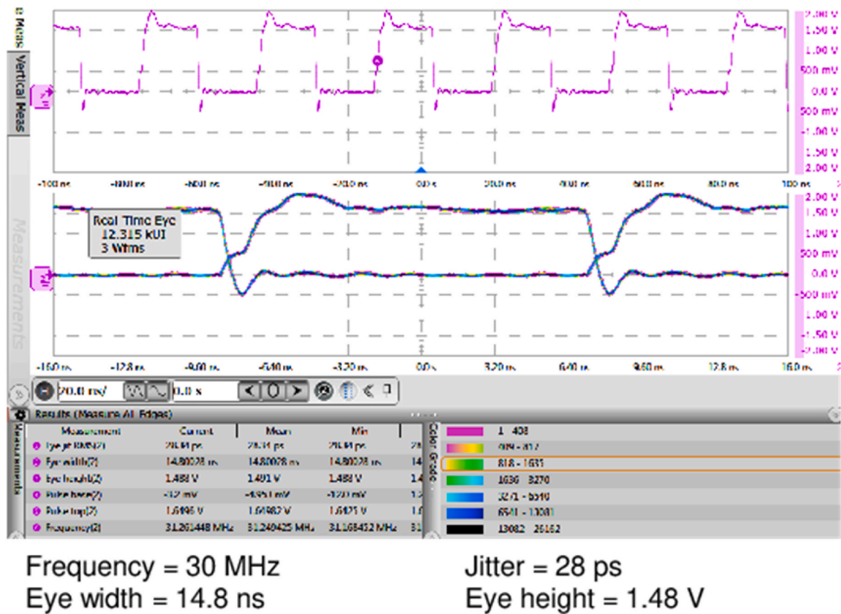
Fig. 22. Output waveform at V_{DD_{ext}} = 1.6 V without PVT detection.
