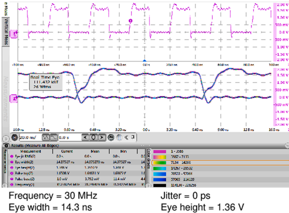
Fig. 23. Output waveform at VDD_{ext} = 1.6 V with PVT detection.
