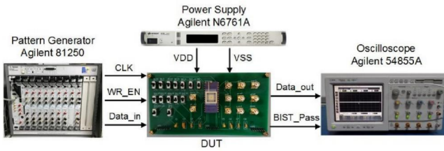
FIGURE 25 Measurement setup for the SRAM prototype
