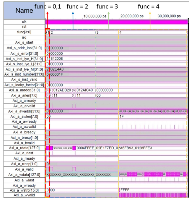
Fig. 18. Pre-layout simulation result after memory scheduling and reorganization by the Reshape module.
