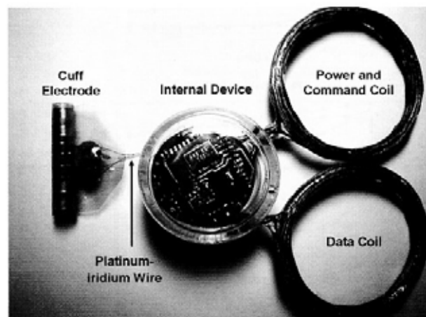
Fig. 7 The implantable wireless biomicrosystem is encapsulated in a glass package with wire connection to cuff electrode.
