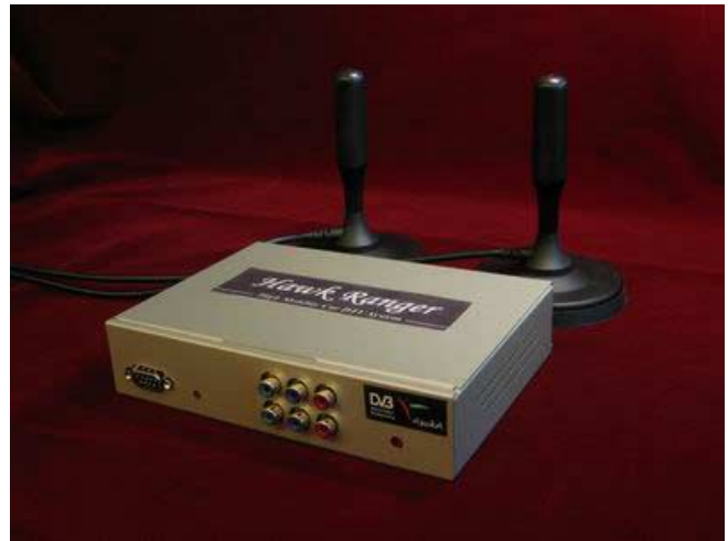
Fig. 6. Outlines of the proposed car-use DVB-T receiver.
